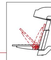
Manually rotate the footrest up and down.
